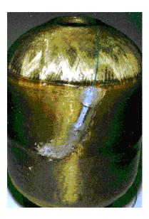
**Figure 1.3:** Optical sensor incorporated in pressure vessel to check the integrity of the vessel.
