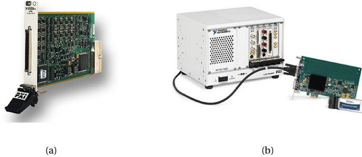
Figure 6.4: PXI driver equipment: (a) PXI 6704 analog output card, (b) PXI 1033 low power chassis.
