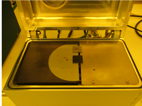
Figure 5.4: Picture of a Unitemp RSS-450-110 hotplate with two samples on it. The black area visible on the left side is the actual hotplate. The samples are sitting on a piece of silicon as a support. The edges of the samples are protruding from the hotplate.
