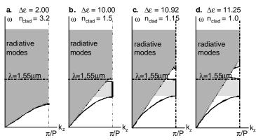
Figure 2: Band structures for different refractive index contrasts.
