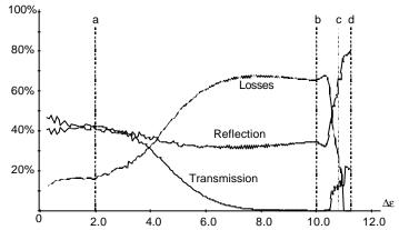
Figure 3: Reflection, Transmission and out-of-plane scattering loss averaged over a structure with 30 to 50 periods.
