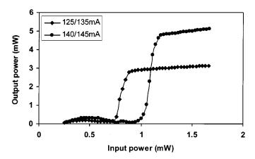
Fig. 2. Measured static decision characteristic for different bias currents to the GCSOAs.
