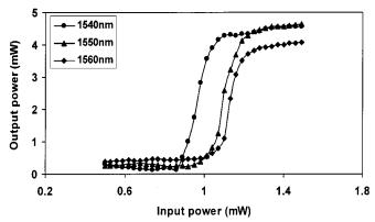
Fig. 3. Regeneration characteristics for different wavelengths, bias currents of two GCSOAs: 135 and 147 mA, respectively.
