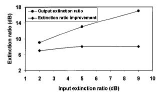
Fig. 5. Output extinction ratio and its improvement as a function of input extinction ratio at 2.488 Gb/s.
