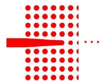
For design purposes it is often desirable to model semi-infinite structures, i.e. structures which are terminated by a semi-infinite crystal. During the design phase we can in this way eliminate parasitic reflections that would come from an imperfect termination of the crystal waveguide. To calculate the reflection matrix of a semi-infinite periodic structure, we first calculate all the Bloch modes of that structure
