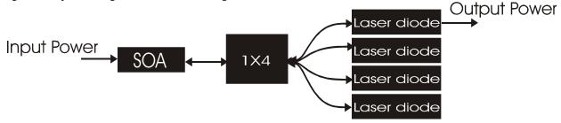
Fig. 2: Schematic of the wavelength-selectable laser used as regenerator
