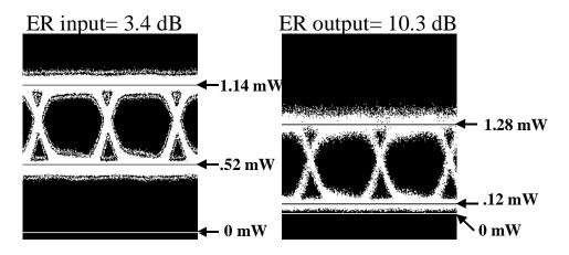
Fig. 4: Input and output eye diagrams
