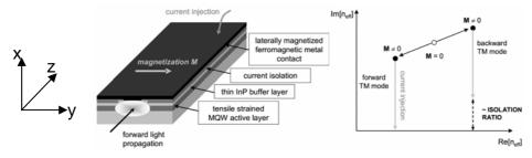
Fig.1 : Schematic representation of the integrated optical isolator and operation principle.
