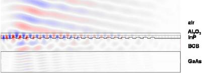
Figure 2. Field profile of a bottom-grating coupler.
