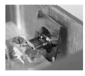
Fig. 2. picture of the fibre pigtailed device. Cleaved chip area is much larger than actually needed.
