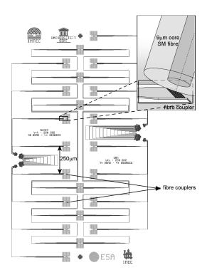
Fig. 1. mask layout with AWG and fibre couplers. Spacing between the couplers is 250 m, compatible with a standard array connector
