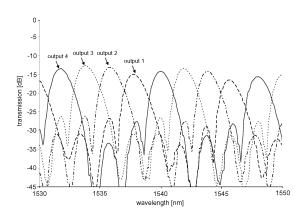
Fig. 3. Fibre to fibre transmission of the pigtailed device, from input 3 to all outputs
