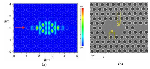
Fig. 1. Photonic crystal micro-cavity. (a) Computed optical field intensity of the resonant mode pattern. The arrow indicates the launching direction of light exciting the resonator. (b) SEM image of the micro-cavity. The period and hole radius are denoted with a and r respectively.
