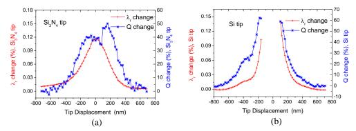
Fig. 5. Nano-mechanical tuning. (a) Change of Q and resonance wavelength detuning for a  $Si_3N_4$  probe versus y-displacement along the scan line shown in Fig. 4(a). (b) The same but now for a Si tip. In close proximity to the field maximum no data could be obtained because the transmission had dropped below the noise level.
