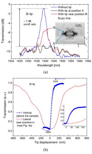
Fig. 4. Nano-mechanical interaction. (a) Transmission spectra for the situation without probe, and with a Si probe positioned at the antinode labeled A, and at a location B close to A, as indicated in the inset. (b) Transmission versus Si tip displacement in the z and y direction [see the dotted "scan line" in the inset of Fig. 4(a)],  $\lambda_s = \lambda_{r,0}$ .
