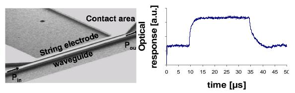
Figure 4: SEM-picture NEMS-device (left) + measurement dynamic optical response (right)
