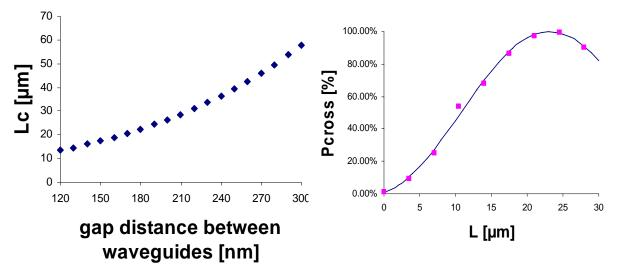
Figure 3: Simulation of Lc in function of g with w=400nm at  $\lambda$ =1.55 $\mu$ m (left); Measurement of P<sub>cross</sub> (squares, right) + theoretical fitting (full line, right) at  $\lambda$ =1.57  $\mu$ m
