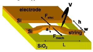
Figure 1: principle of electrostatic actuation
