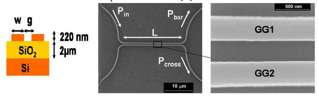
Figure 2: directional coupler: cross-section (left), SEM-picture + detail (right)
