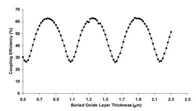
**Fig. 1**: Coupling efficiency of a silver grating coupler (period = 610 nm, fill factor = 30 %, height = 20 nm) as a function of buried oxide layer thickness.
