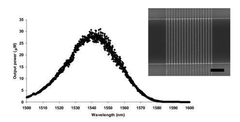
Fig. 2: Measurement data of fiber-to-fiber transmission via two gold grating couplers on top of a 10 μm wide SOI waveguide. Input power is set to 1 mW. Inset: SEM-picture of a gold grating coupler prototype. Bar length is 3 μm.
