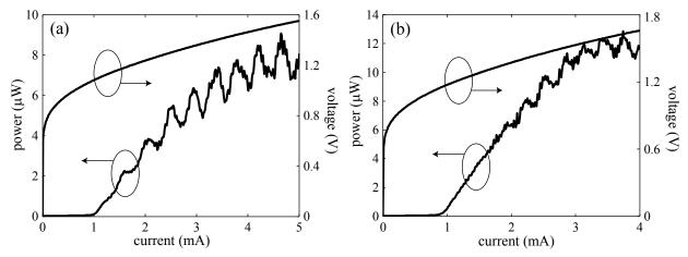
Fig. 2. LIV curves of microdisk lasers with (a) 10µm diameter and (b) 7.5µm diameter under CW. Powers were normalized by the efficiency of the grating coupler.
