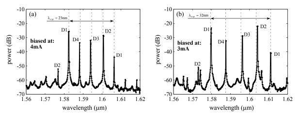
Fig. 3. Normalized spectra of the MWLs from the left end of the bus SOI waveguide when the four microdisk lasers were simultaneously biased at the same current, (a) for 10 $\mu$ m diameter group and (b) for 7.5 $\mu$ m diameter group. The dashed lines are separated by  $\lambda_{FSR}/4$ . The corresponding disk number is marked on each of the laser peaks (cf., Fig. 1).
