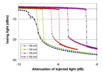
Figure 2: Measured bistability for a  $\lambda$ /4-shifted DFB-laser of 400  $\mu$ m and different injection currents.
