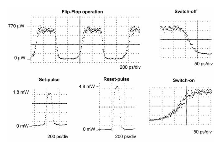
Figure 3: All-optical flip-flop operation using pulses of 100 ps with energy less than 0.5 pJ. Repetition rates up to 1.25 GHz can be obtained and the switch-on time of the laser is only 120 ps.
