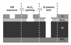
Figure 1. Schematic overview of the three-step process flow. In the first step  $Al_2O_3$  acts as etch stop layer and protects the silicon, in the final step  $Al_2O_3$  is again etched slowly and acts as hard mask.
