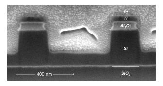
Figure 3. Cross-section micrograph of fabricated 400 nm wide and 150 nm deep trenches in the top 220 nm silicon layer of a silicon-on-insulator. Some Ti is still visible on top of the  $Al_2O_3$ .
