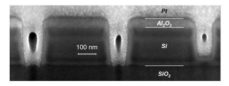
Figure 2. Cross-section micrograph of fabricated 100nm wide slits in the top 220 nm silicon layer of a silicon-on-insulator substrate. Pt was deposited in the slits to keep them intact while making the cross-section with FIB.
