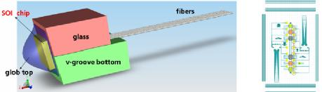
Figure 2 (a) Fiber array based package for Silicon photonic chip (SOI chip). Stability of the package is based on the actual fiber array mount, which consists of a V-groove bottom & a glass lid. The SOI chip contains a number of equally spaced grating couplers (optical i/o-ports). An example of a corresponding layout is shown in (b). The couplers are indicated by the circles shaded in color.
