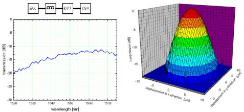
Figure 5: (a) Wavelength dependence of transmission through 2 shortened grating couplers. (b) Transmission characteristic of fiber-to-grating coupler in the dependence of lateral displacement.
