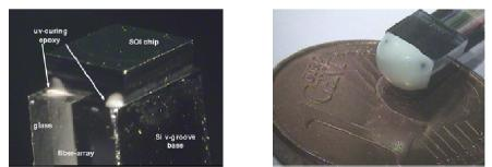
Figure 4: (a) Fiber array based package without glob top. The SOI chip is mounted face down on the fiber array. (b) Encapsulated SOI chip on fiber array (8 fibers) in comparison to 1 Euro Cent coin.
