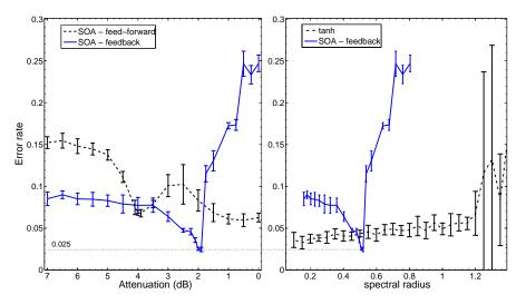
Fig. 5. Results with a signal frequency of  $0.5 \,\text{GHz}$ , simulation time: 100 ns, amplitude power:  $5 \,\text{mW}$ , delay:  $6.25 \,\text{ps}$ ,  $25 \,\text{nodes}$ : (left) – photonic reservoirs with and without feedback, (right) – classical reservoirs versus photonic reservoirs with feedback
