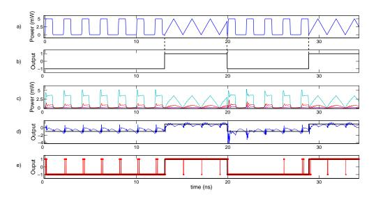
Fig. 4. Pattern recognition task: a) Input signal with different transitions between the rectangular and triangular waveform b) desired output c) state (i.e. optical power level) of some of the reservoir nodes d) The approximation (blue) of the desired output (black) by the readout function, e) final output of the system (red)
