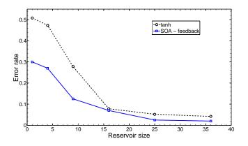
Fig. 6. This figure shows the influence of the reservoir size on the performance of the classical and photonic reservoirs with feedback.
