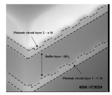
Fig.2 SEM Cross-section view showing the grating coupler in the bottom and top photonic circuit.
