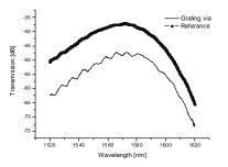
Fig. 3 Transmission spectrum of a grating optical via **3. SUMMARY**
