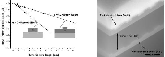
Figure 1 (left) Propagation loss of a silicon photonic wire (480X220nm) and a shallow etched ridge waveguide and (right) Optical Via to couple light from one photonic layer to other.
