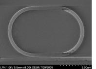
Figure 1. SEM image of racetrack resonators
