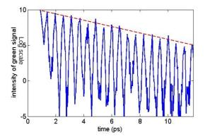
Figure 2. The intensity of the signal measured at 540nm (log scale) vs the delay time of the pump. The temporal ring-down of the racetrack shown as a sequence of diminishing peaks.
