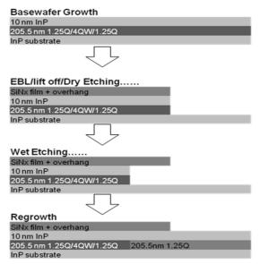
Figure 2. Fabrication process flow
