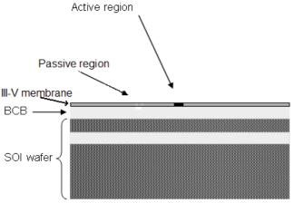
Figure 1. Schematic of InP membrane on SOI platform
