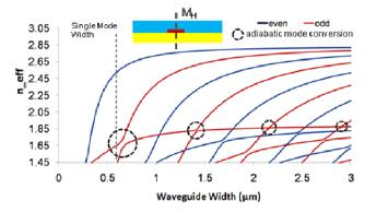
Figure 2. Adiabatic Mode Profile of an asymmetric waveguide.
