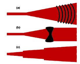
Figure 3. Non-Adiabatic tapers: (a) Focusing Grating Coupler (b) Lensed Focusing Taper (c) Discontinuous Taper
