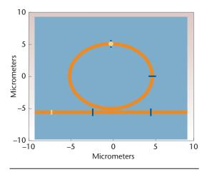
Figure 1. The automatic visualization of a 2D simulation landscape based on Python-Meep and Matplotlib. This visualization shows a ring resonator with access waveguide in silicon (orange), the position of the source (tan line), two fluxplanes (blue lines), and a probing point (tan circle).
