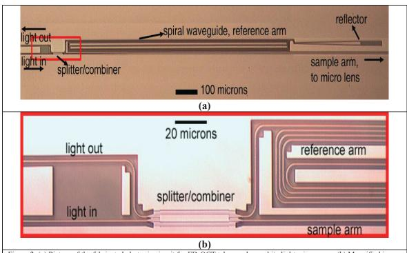
Figure 2. (a) Picture of the fabricated photonic circuit for FD-OCT taken under a white light microscope. (b) Magnified image of the area marked with a red rectangle.
