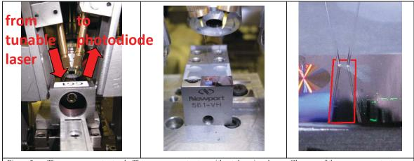
Figure 3. a. The measurement setup b. The measurement setup without the micro lens c. Close up of the measurement setup, the structure is located in the red rectangle, input and output fibers are clearly shown.
