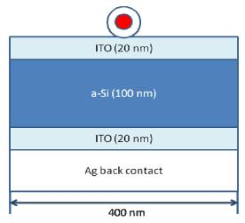
Fig. 1. A cross-section of the investigated SC. (ITO stands for indium tin oxide).
