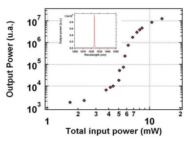
Figure 2. Light-Light curve of laser emission (log-log scale)
