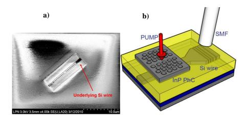
Figure 1. Saturated SEM image showing the Si wire beneath the III-V cavity and schematic of cavity aligned to wire.
