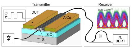
Figure 3: Data transmission experiment: Laser light is launched into the SOH slot waveguide, and an electrical 42.7 Gbit/s signal is fed to the electrodes. This generates a purely phase-modulated signal. On the receiver side, phase-to-amplitude conversion is achieved by feeding the signal into a delay interferometer (DI) that superimposes optical waves from subsequent bit slots. DUT = device under test, BERT = bit-error ratio tester
