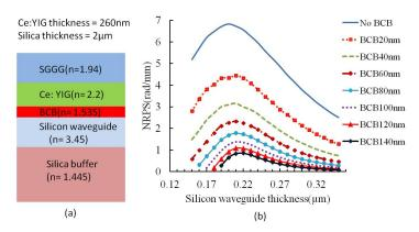
Fig. 1. (a) Slab waveguide stack and (b) simulation of the nonreciprocal phase shift as a function of silicon waveguide thickness and DVS-BCB bonding layer thickness.
