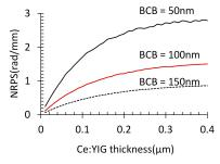
Fig. 5. Nonreciprocal phase shift as a function of Ce:YIG layer thickness for a 220nm thick silicon waveguide layer thickness and different DVS-BCB bonding layer thicknesses.
