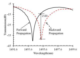
Fig. 9. Normalized MZI transmission spectra for forward and backward propagation.
