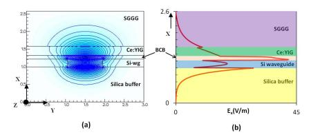
Fig. 3. (a) Contour plot of  $E_x^0$  field of the quasi-TM polarized mode (b) field enhancement in the DVS-BCB bonding layer due to a vertical slot waveguide effect.
