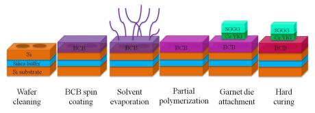
Fig. 6. Schematic illustration of the bonding procedure.
