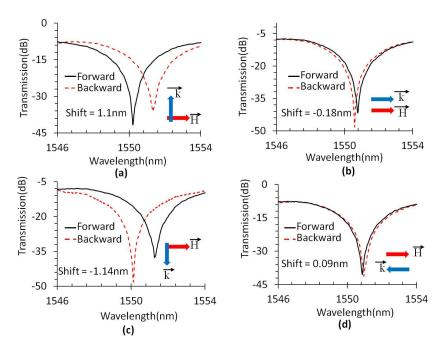
Fig. 10. Normalized transmission spectra of the MZI for different angular orientations of magnetic field with respect to the light propagation direction: (a)  $90^{\circ}$ , (b)  $0^{\circ}$ , (c)  $270^{\circ}$ , (d)  $180^{\circ}$ .
