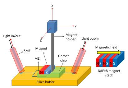
Fig. 8. Schematic diagram of measurement set up and magnet stack.
