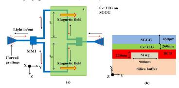
Fig. 4. Schematic of the proposed optical isolator consisting of a Mach-Zehnder interferometer covered by Ce:YIG; (a) top view and (b) cross- section view.
