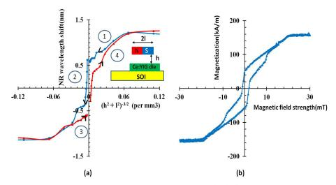
Fig. 11. (a) Nonreciprocal wavelength shift as a function of  $(h^2 + l^2)^{-3/2}$ , where h is the distance between the magnet and the Ce:YIG layer and 2l is the distance between the two poles of the magnet stack. Negative values for  $(h^2 + l^2)^{-3/2}$  indicate that the magnet was rotated 180 degrees, (b) magnetization curve of the Ce:YIG layer after subtracting the contribution from the paramagnetic SGGG substrate.
