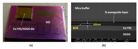
Fig. 7. Photograph of the Ce:YIG/SGGG die bonded to an SOI waveguide circuit (a) and an SEM cross-section image of the bonded stack (b).
