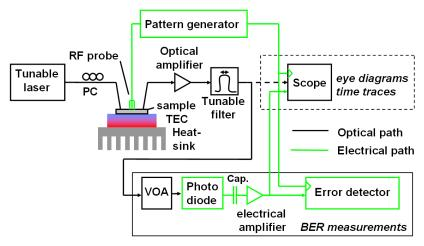
Fig. 3. Measurement apparatus for high-speed measurements (eye diagrams and bit-error rate test).
