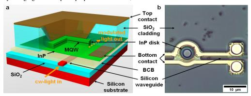
Fig. 1. Device structure of an InP microdisk modulator heterogeneously integrated on a SOI waveguide. a) Schematic view of the final device including the final metalization. b) Optical microscope image of the InP microdisk modulator before the final pad metallization.
