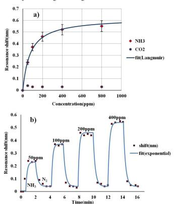
Fig. 2. response from a microporous acidic film coated MRR (a) resonance shift with respect to NH3 and CO2 concentrations (b) response and recovery with time at NH3 concentrations of 50,100,200 and 400 ppm introduced for two minutes.
