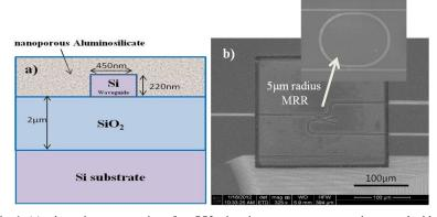
Fig. 1. (a) schematic representation of an SOI microring resonator cross section coated with a porous gas sensitive film (not drawn to scale) (b) Scanning Electron Micrograph of a  $5\mu$ m radius MRR coated by a mesoporous silica film (thickness ~100 nm);Inset:magnified view of the coated MRR.
