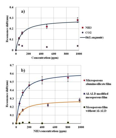
Fig. 3. (a) measured response from mesoporous silica coated MRR upon saturation with  $NH_3$  and CO2 gases, (b) comparison of  $NH_3$  sensitivity of microporous aluminosilicate film, and mesoporous silica film with and without Al-ALD
