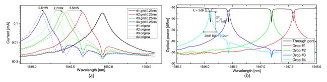
Fig. 3: The 4-channel demultiplexer (a) optical to optical response of the TM-strip approach (b) the optical-electrical TE-rib approach with channels tuned on a 0.25nm grid with -15dB XT
