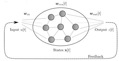
Figure 1. Principle of FORCE: The output of the reservoir is fed back to the input. During training, the output weights  $w_{out}[t]$  are modified using the RLS rule which is described below.
