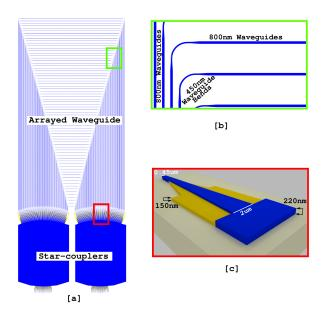
Fig. 3. (a) Mask layout of silicon AWG. (b) Zoom into waveguide array region, showing combination of 450nm and 800nm wide waveguides to minimize phase errors. (c) A  $2\mu m$  wide shallow etched aperture.
