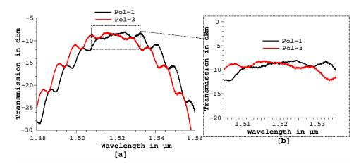
Fig. 6. Transmission of two 2-D grating couplers connected through waveguides. (a) Spectral response of the 2D grating for wavelength rage of  $1.48\mu m$  to  $1.56\mu m$ . (b) Flat passband spectral response of the 2D grating.
