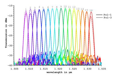
Fig. 7. Spectral response of a 16 channels 200GHz polarization diversity wavelength demultiplexer circuit for Pol-1 and Pol-3 polarizations.
