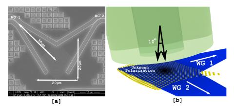
Fig. 2. (a) Fabricated 2D grating coupler. (b) Schematic diagram of a 2D grating coupler with fiber align.
