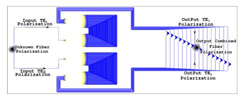
Fig. 1. Schematic diagram of  $16 \times 400 GHz$  Polarization diversity circuit.
