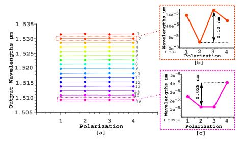
Fig. 8. (a) The output wavelength channel positions of the polarization diversity circuit for Pol-1, Pol-2, Pol-3, and Pol-4 polarizations. (b) Maximum shifted output channel. (c) Minimum shifted output channel.
