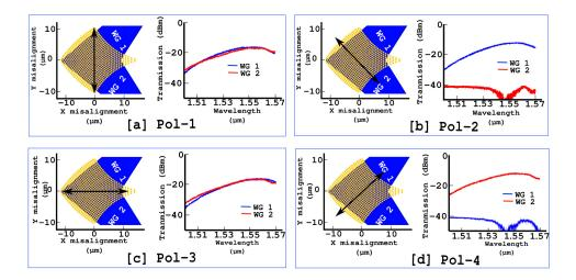
Fig. 4. Spectral response of a 2D grating coupler connected to two 1D grating couplers for differently oriented input polarizations ((a) Pol-1: 90 degree, (b) Pol-2: -45 degree, c) Pol-3: 0 degree, (d) Pol-4: 45 degree oriented fiber polarizations with respect to the axis of the 2D grating).
