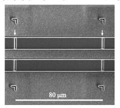
Figure 2. The apparent overlap after stitiching is found almost entirely to the right of the stitch line (white arrows), indicating that the edge rate is faster near the edge of the previous rectangle.
