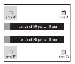
Figure 1. Scheme for stitching, indicating structures to etch (black), areas to image (light grey) and previously etched structures (dark grey).
