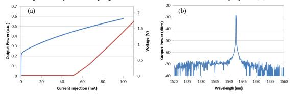
Fig. 4. (a) The L-I-V curve for a single mode laser ;(b) Lasing spectrum of the hybrid single mode laser for 80mA current injection at 20°C
