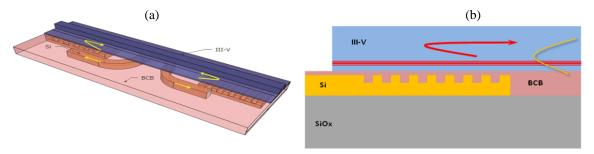
ig. 1. (a) Schematic of the active DBR with the evanescent coupling waveguide in the center of the laser cavity (b) schematic view of a hybrid DBR reflector in the hybrid silicon laser.
