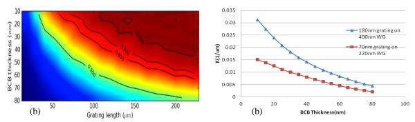
Fig. 2. (a) Grating reflection as a function of the number of grating periods and DVS-BCB thickness (b) Coupling constant  $\kappa$  for a hybrid grating simulated for different grating cross-sections versus DVS-BCB thickness.
