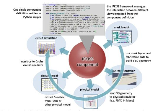
Fig 2.: Principle of the IPKISS parametric design framework. Views are derived from a single component definition, and the information can be handed over automatically between views.
