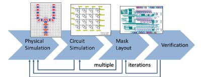
*Fig. 1: Aspects of typical photonic design. While the basic design flow should proceed from left to right, in practice it requires multiple iterations which force the designer to go back to earlier stages (and tools).*
