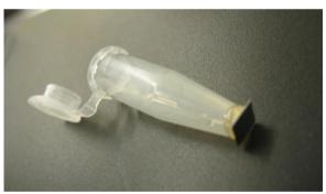
Figure 5. Silicon photonic chip with the array of sensors and the embedded microfluidic system incorporated in the bottom of a reaction tube.
