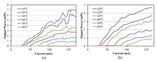
Fig. 5. Output power as a function of current for different stage temperatures for the RMFL (a) and AMFL (b). Lasing up to temperatures of  $60^{\circ}$ C is obtained in both cases.
