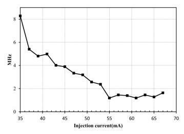
Fig. 6. Linewidth measurement of the ring-resonator based multi-frequency laser
