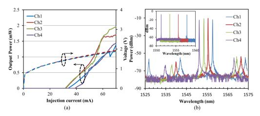
Fig. 4. a) LIV curves for the ring based demultiplexer. The output power refers to the amount of light coupled in the silicon waveguide b) Superimposed spectra for the 4 channels (resolution bandwidth 0.1 nm). The inset shows the spectra measured with a resolution bandwidth of 0.2 pm.
