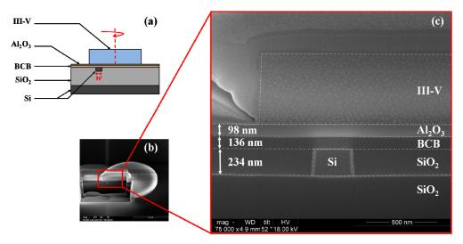
Fig. 2. (a) Schematic of microdisk cross-section (cylindrical revolution along the dashed line). (b) SEM image of the location of the cross-section on a microdisk laser. (c) SEM image of the cross-section of a lasing device coupled to a 300nm-wide waveguide.
