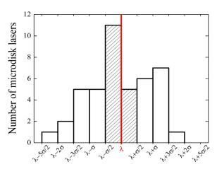
Fig. 8. Wavelength distribution of 43 microdisk lasers of the same sample centered on  $\lambda$ . The patterned area shows that the peak lasing wavelength of 16 microdisk lasers is between  $\lambda$ - $\sigma$ /2 and  $\lambda + \sigma$ /2
