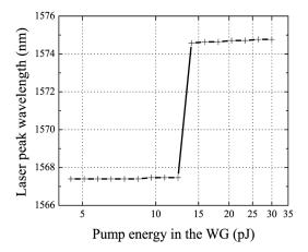
Fig. 5. Mode competition in 7- $\mu$ m diameter microdisk laser optically pumped through the waveguide at 1.18 $\mu$ m.
