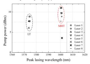
Fig. 9. Laser threshold (LT) and mode hopping threshold (MHT) in nominally identical microdisk lasers under increasing pump power.
