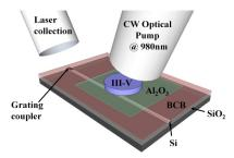
Fig. 6. Schematic of optical pumping of a microdisk laser from the top surface.
