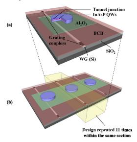
Fig. 1. Schematic of the sample. (a) Microdisk laser structure coupled to underlying waveguide. (b) Array of nominally identical microdisk lasers.
