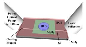
Fig. 3. Optical pumping of a microdisk through the underlying Si waveguide.
