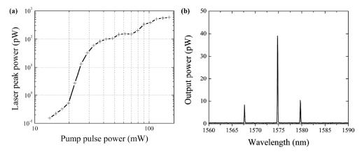
Fig. 4. (a) S-shape curve of a 7- $\mu$ m diameter microdisk laser optically pumped through the waveguide at 1.18 $\mu$ m (log-log scale). (b) Measured lasing spectrum of the microdisk under 30pJ of pump energy.
