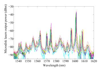
Fig. 7. Spectra of 9 nominally identical microdisk lasers processed with electron-beam lithography and optically pumped at 980nm. The standard deviation in peak lasing wavelength is 0.37nm.
