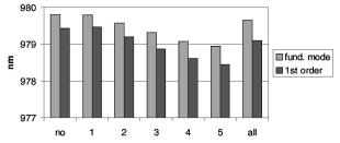
Fig. 10. Lasing wavelength (oxidized VCSEL): 1, node oxide; 5, antinode oxide; no, no oxide; all,  $\lambda/4$  oxide.
