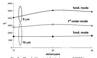
Fig. 6. Threshold material gain (airpost VCSEL).
