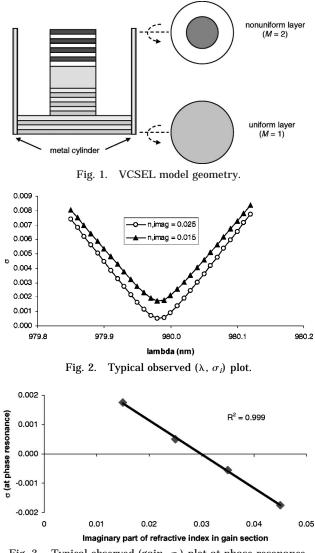
Fig. 3. Typical observed (gain,  $\sigma_i$ ) plot at phase resonance.
