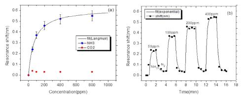
Figure 1 Response from a microporous acidic film coated MRR (a) resonance shift with respect to  $NH_3$  and  $CO_2$  concentrations (b) response and recovery with time at  $NH_3$  concentrations of 50,100,200 and 400 ppm introduced for two minutes.
