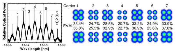
**Fig. 3:** Data transmission results: Data transmission of 784 Gbit/s using QPSK signals on 7 carriers generated by an integrated SOH comb source. Comb spectrum (left) and constellation diagrams for all channels and both polarization are depicted along with measured EVM values. BER below hard-decision threshold are achieved for all signals.
