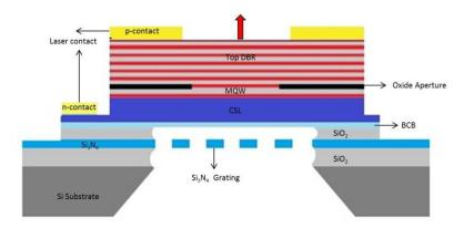
Figure 3. Schematic cross-sectional view of the VCSEL, consisting of a half VCSEL on top of a free-standing Si<sub>3</sub>N<sub>4</sub> grating.
