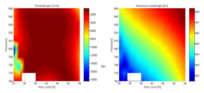
Figure 5. Resonant half-VCSEL design case. (left) Threshold gain as function of grating period and DC, and (right) gresonance wavelength as function of grating period and DC.
