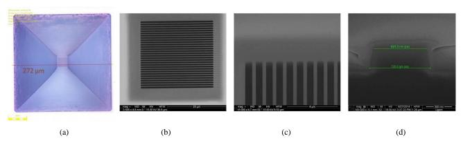
Figure 7. Fabricated free standing  $Si_3N_4$  grating (a) Microscopic image taken from the backside of the Si wafer (b) SEM image taken from the top of the grating. (c) a  $52^{\circ}$  tilted SEM view of the grating (d) cross-sectional SEM view of the  $Si_3N_4$  waveguide showing the topology of the grating bars.
