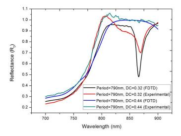
Figure 8. Measured and simulated reflection spectra from a Si<sub>3</sub>N<sub>4</sub>-based HCG.
