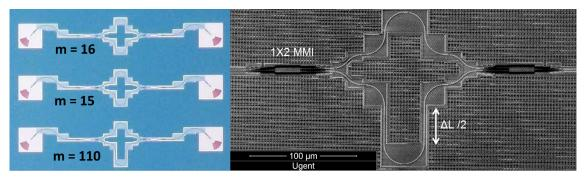
Fig. 1: (a). Camera image of fabricated devices and (b) SEM image of fabricated MZI with m =110.
