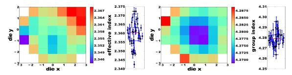
Fig. 4: Wafer statistics and map at 1550 nm (a)  $n_{eff}$  and (b)  $n_g$
