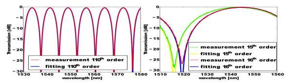
Fig. 2: Measured and fitted normalized spectrum of MZI (a) higher filter order and (b) lower filter order.
