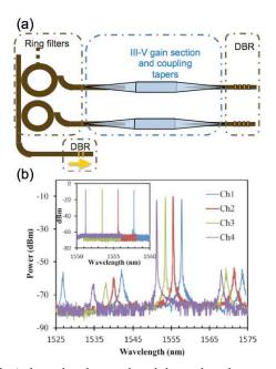
Figure 2: 4-channel multi-wavelength lasers based on ring-resonator intra-cavity filter elements: (a) layout; (b) optical output spectrum
