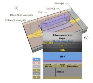
Figure 1: (a) layout of III-V on silicon DFB laser with the first order grating defined in the silicon waveguide layer; (b) SEM cross-section of the III-V-on-silicon laser structure
