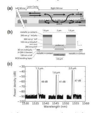
*Figure 4: Resonant cavity mirror laser: (a) layout; (b) emission spectrum*
