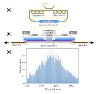
Figure 3: ring-cavity mode-locked laser geometry (a); longitudinal cross-section indicating the SOA and SA sections (b) and the generated optical output spectrum (c).
