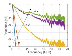
Fig. 5. Normalized frequency response (S<sub>21</sub>) of a  $3 \times 10 \,\mu$ m<sup>2</sup> UTC-PD measured at different bias voltages.
