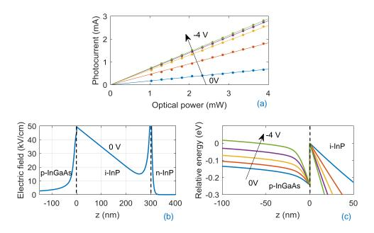
Fig. 4. (a) Bias dependent photocurrent versus optical power coupled to the UTC-PD. (b) Simulated electric field distribution in the vertical direction of the UTC-PD at zero bias and 1 mA photocurrent. (c) Simulated conduction band discontinuity at the InGaAs/InP interface.
