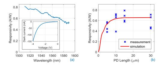
Fig. 3. (a) Responsivity versus wavelength of a  $3 \times 10 \ \mu m^2$  UTC-PD measured at -4 V; the inset shows the measured dark current versus bias voltage . (b) Responsivity as a function of the length of the UTC-PDs. Both measurement data and simulation results are shown.
