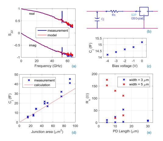
Fig. 6. (a) Real part and imaginary part of the reflection coefficient ( $S_{22}$ ) of a  $3 \times 10 \ \mu m^2$  UTC-PD. Results from measurements and modeling are both shown. (b) The equivalent circuit model of the UTC-PD. (c) Bias dependence of the junction capacitance ( $C_j$ ) extracted from the model. (d)  $C_j$  of different UTC-PDs as a function of the junction area. (e) Series resistance ( $R_s$ ) of different UTC-PDs versus their length.
