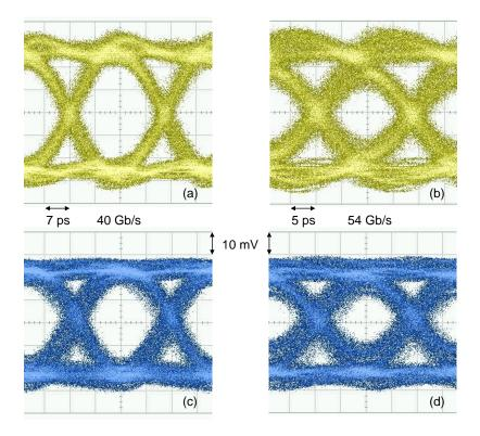
Fig. 7. Reference optical eye diagrams output from the commercial modulator at (a) 40 Gb/s and (b) 54 Gb/s, along with the associated electrical eye diagrams output from the  $3 \times 10 \ \mu\text{m}^2$  UTC-PD at (c) 40 Gb/s and (d) 54 Gb/s.
