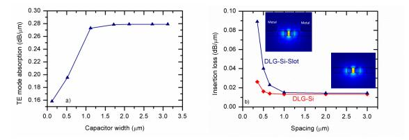
Figure3. a) The TE mode absorption at Dirac point for the scattering time of 65 as function of capacitor width b) The insertion loss as function of the distance of metal edge and the waveguide edge (spacing). In the case of DLG-Si-Slot, the total waveguide width is 520 nm.
