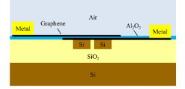
Figure1. A schematic of the double layer graphene-on-Si slot waveguide optical switch.
