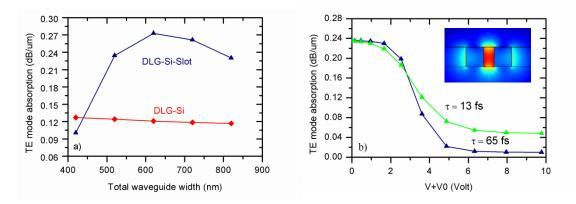
Figure 2. a) The TE mode absorption at the Dirac point versus the total waveguide width (2×Si section width + slot section width), the graphene scattering time is 65 fs b) The TE mode absorption for the
