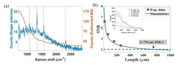
Fig. 2 (a) The Raman spectra measured from a waveguide functionalized with a single N=1 antenna (blue). The background spectrum is shown on the right axis. (b) The measured and fitted Signal-to-noise ratio for a single antenna on waveguides of length L. The small inset shows the Raman spectra for waveguides of L=20,70,160 and  $260\,\mu m$ .
