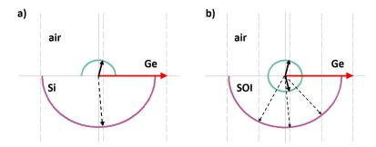
Fig. 2. Vector diagram of a second order Ge-on-Si grating (a) and a fourth order Ge-on-SOI grating (b) with the buried oxide layer locally removed. The allowed diffraction orders in air (solid arrows) and Si under-cladding (dashed arrows) are also indicated.
