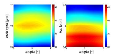
Fig. 5. Maximum coupling efficiency in the 5-5.6  $\mu$ m wavelength range for the Ge-on-Si grating coupler as a function of the grating etch depth and fiber angle (a) and as a function of thickness of the Ge layer and fiber angle (b).
