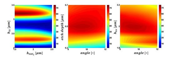
Fig. 7. Maximum fiber-to-chip coupling efficiency in the 5 to 5.6  $\mu$ m wavelength range for the Ge-on-SOI grating coupler depending on different parameters: Si and SiO<sub>2</sub> layer thickness (a), grating etch depth and fiber angle (b) and the thickness of the Ge waveguide layer vs. fiber angle (c).
