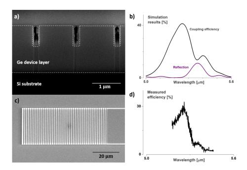
Fig. 4. Cross-section (a) and top view of the optimized Ge-on-Si grating coupler (c). Simulation (b) and measured data of the same device (d).
